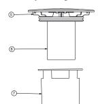
Insert the container and trap (6-7) firmly engage the trap in the bottom position
